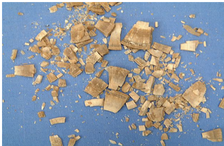
Figure 9. Scale removed by using three nozzles
