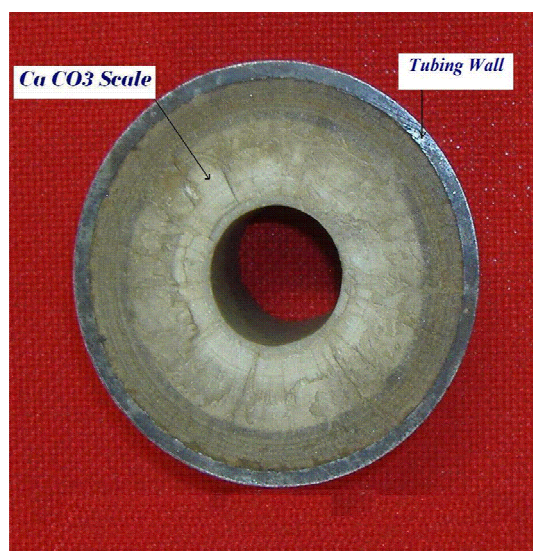
Figure 2. Scale formation in the production tubing.
